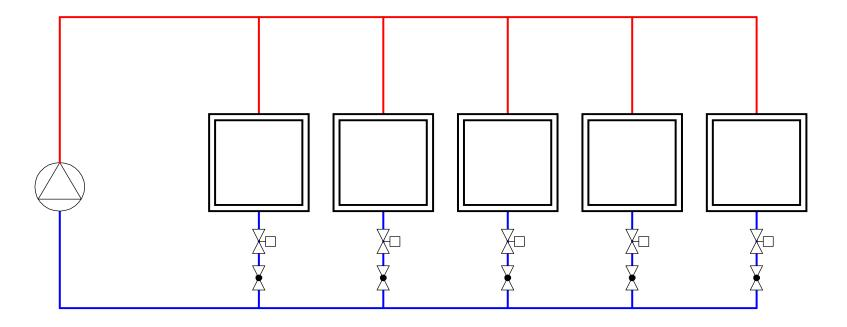
Balancing values are required, as well as initial balancing of the system. Flows are constantly changing as a result of the fluctuation of the  $\Delta P$  due to control values constantly opening and closing and pump speeds ramping up and down.
