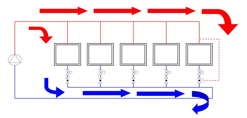
Will provide even flows without the use of balancing valves and having to balance the system, but it involves more engineering time plus more material and more upfront installation costs than direct return piping. Valves are still constantly opening and closing unnecessarily as a result of fluctuating system dynamics, which still results in unstable flows and lower  $\Delta$ Ts, especially at low loads.
